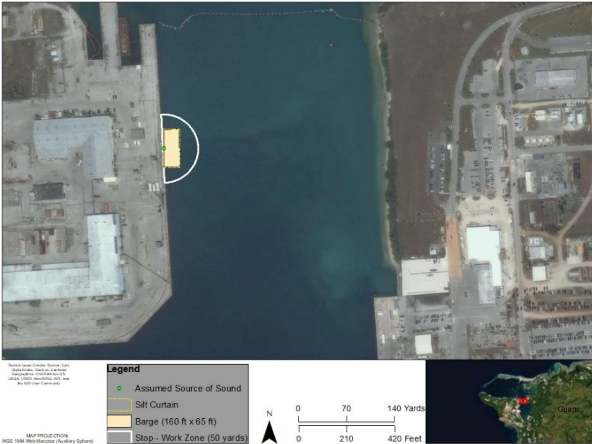
Figure 9. Representation of the in-water Action footprint, including the approximate locations of the barge, silt curtain, and the 50-yard shut-down zone.
